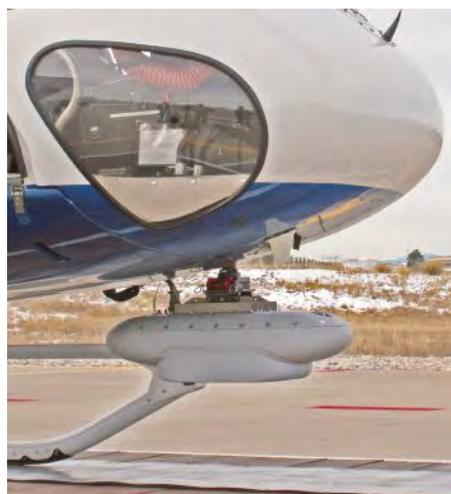
WAMI sensors can support 10 field operators at once, each able to open streaming video windows to watch a different area within the sensor's 2.5 mile-wide field of view. Leveraging focal planes developed for medical imaging, these systems can cost less than \$1 million a unit.
